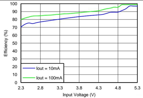
Figure 10. Efficiency vs Input Voltage
