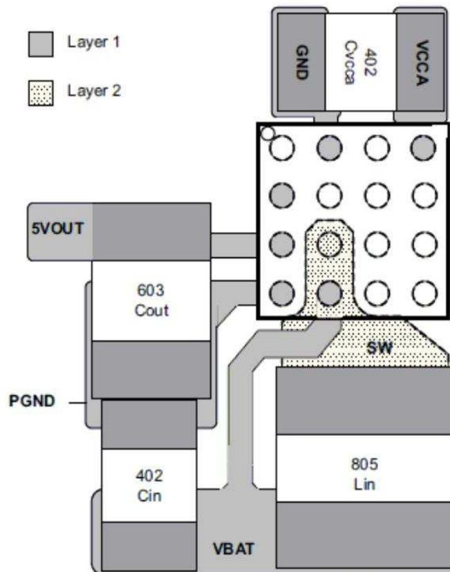
**Figure 17. Board Layout With DC-DC Components (Top View)**
