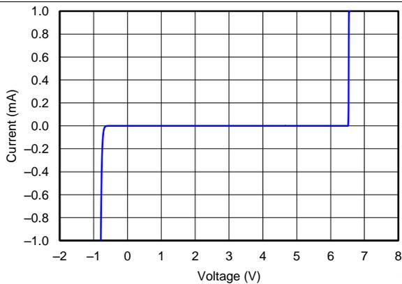
Figure 5. DC SWEEP V-I Curve
