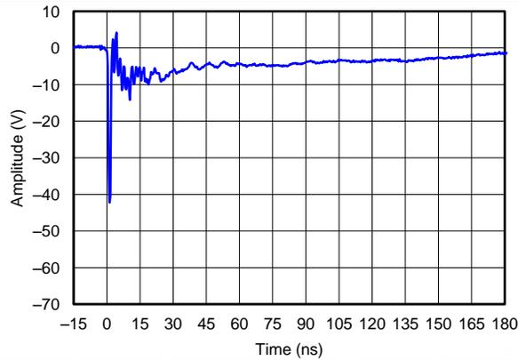
Figure 7. IEC 61000-4-2 Clamping Voltage, -8-kV Contact
