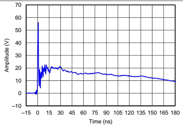
Figure 6. IEC 61000-4-2 Clamping Voltage, 8-kV Contact
