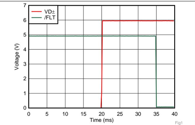
Figure 13.  $\overline{FLT}$  Assertion Time During OVP
