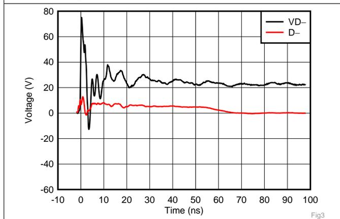
Figure 4. 8-kV ISO 10605 (330-pF, 330-Ω) Contact Waveform
