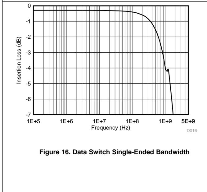
Figure 16. Data Switch Single-Ended Bandwidth
