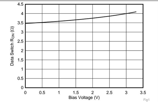
Figure 11. Data Switch  $R_{ON}$  vs Bias Voltage
