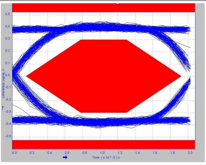
Figure 23. USB2.0 Eye Diagram (System from Typical Application Schematic)
