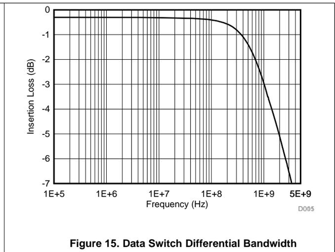
Figure 15. Data Switch Differential Bandwidth
