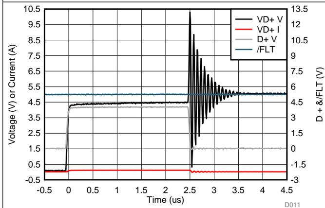
Figure 12. Data Switch Short-to-5 V Response Waveform
