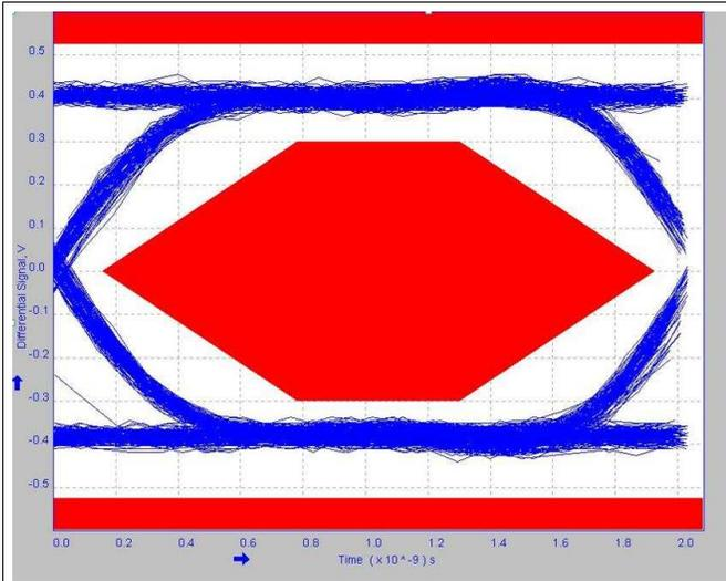
Figure 22. USB2.0 Eye Diagram (Board Only, Through Path)
