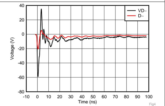
Figure 5. -8-kV ISO 10605 (330-pF, 330-Ω) Contact Waveform
