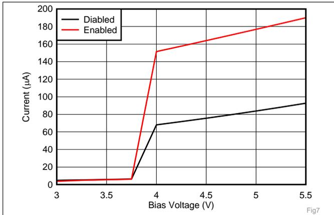
Figure 8.  $V_{PWR}$  Operating Current vs Bias Voltage
