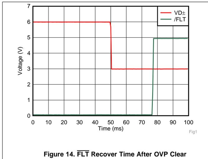
Figure 14.  $\overline{FLT}$  Recover Time After OVP Clear
