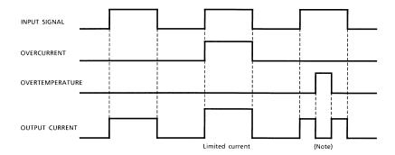
Note: The overtemperature detector circuits feature hysteresis. After overtemperature is detected, normal operation is restored only when the junction temperature falls by the hysteresis amount (10°C typ.) in relation to the overtemperature detection temperature.
