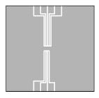
Glass epoxy board Material : FR-4 25.4mm × 25.4mm × 0.8mm (b) Glass epoxy board
