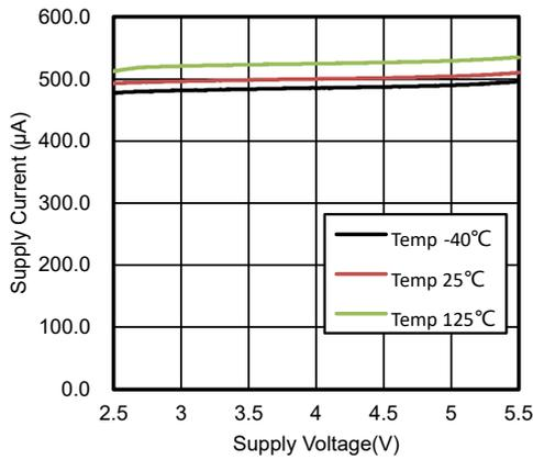
Figure 1. Supply Current vs. Supply Voltage, Output High
