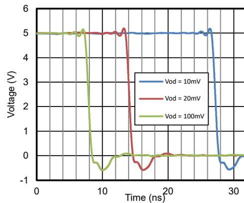
Figure 2. Propagation Delay, High to Low
