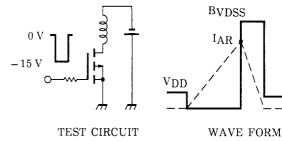
$$\begin{array}{l} T_{ch}\!=\!25^{\circ}\!C\:(Initial) \\ Peak\:\:I_{AR}=-5\:A,\:R_{G}=25\:\Omega \end{array}\:\:E_{AS}=\frac{1}{2}\cdot L\:\cdot I^{2}\cdot\:(\frac{B_{VDSS}}{B_{VDSS}-V_{DD}}\:)\:\:V_{DD}=-24\:V,\:L=1.0\:mH \end{array}$$
