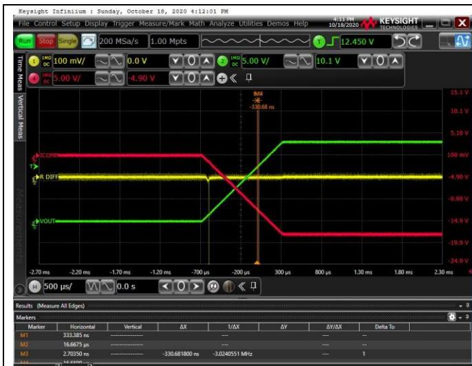
Figure 23. 1ms Power On and Off Time
