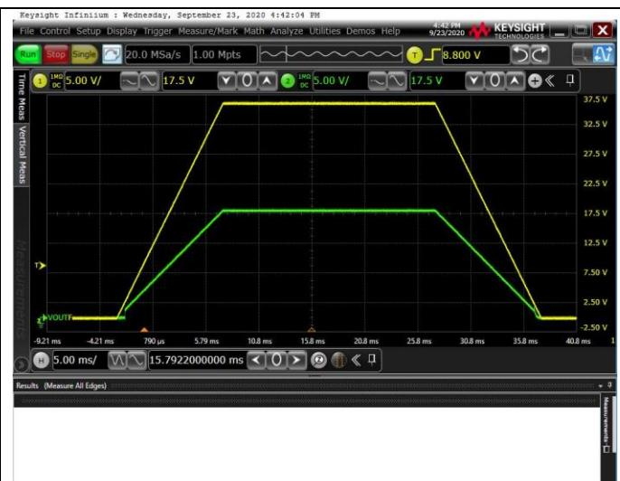
Figure 20. 10ms Power On and Off Time
