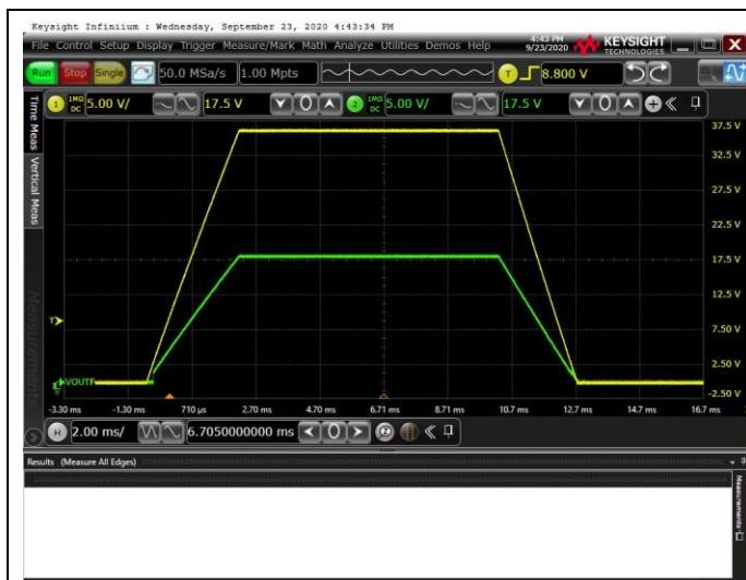
Figure 19. 2ms Power On and Off Time
