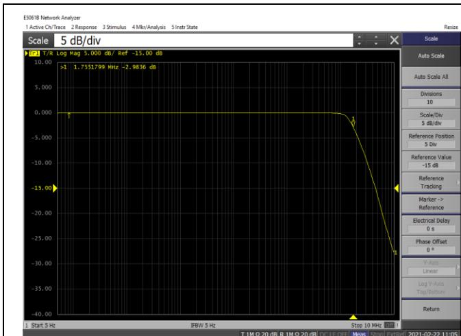
Figure 7. -3dB Bandwidth,  $G = 1$ ,  $V_s = 30V$
