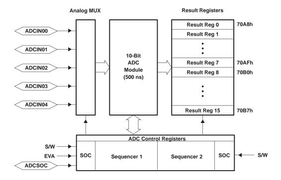
Figure 15. Block Diagram of the 2401A ADC Module
