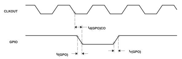
Figure 36. General-Purpose Output Timing
