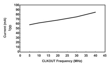
Figure 21. LF2401A Typical Current Consumption (With Peripheral Clocks Enabled)
