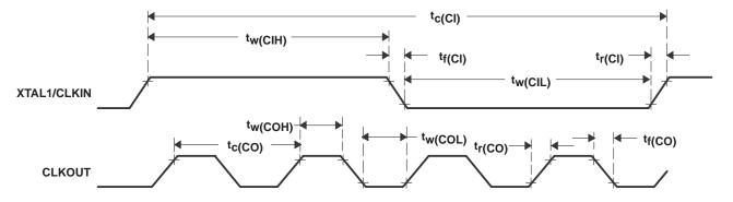
Figure 25. CLKIN-to-CLKOUT Timing With PLL and External Clock in ×4 Mode
