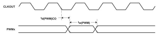
Figure 33. PWM Output Timing
