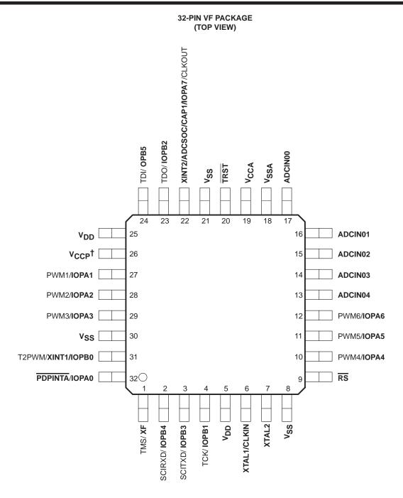
† Pin 26 is V<sub>CCP</sub> on LF2401A and is a No Connect (NC) on LC2401A. NOTE A: Bold face type indicates function of the device pin after reset.
