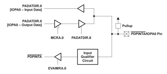
Figure 2. PDPINTA/IOPA0 Pin Multiplexing Functional Block Diagram
