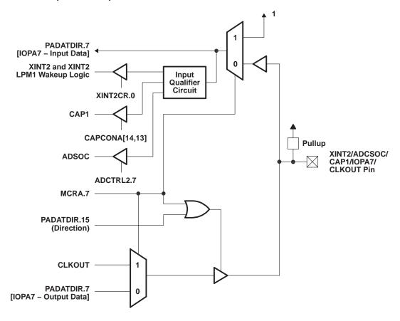
Figure 3. XINT2/ADCSOC/CAP1/IOPA7/CLKOUT Pin Multiplexing Functional Block Diagram
