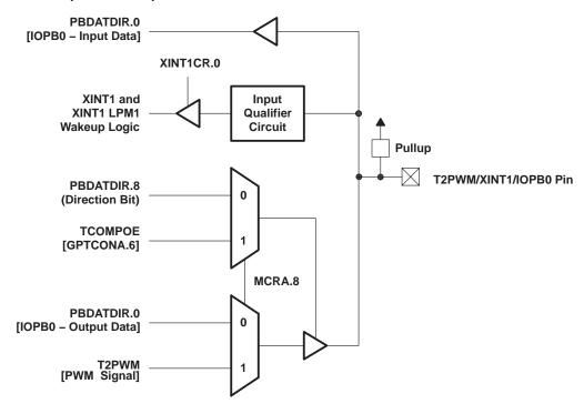
Figure 4. T2PWM/XINT1/IOPB0 Pin Multiplexing Functional Block Diagram
