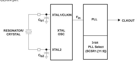
Figure 17. PLL Clock Module Block Diagram
