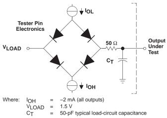
Figure 22. Test Load Circuit
