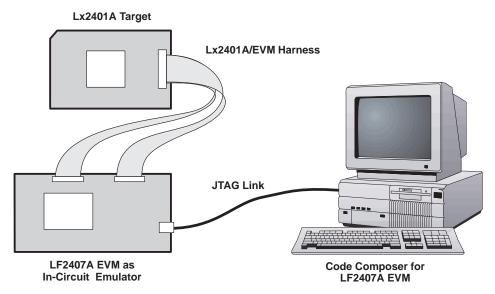
Figure 8. Lx2401A Emulation Using LF2407A EVM as In-Circuit Emulator (Optional)
