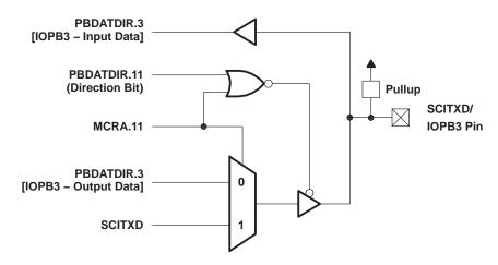
Figure 5. SCITXD/IOPB3 Pin Multiplexing Functional Block Diagram
