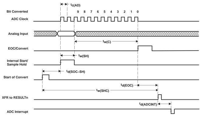
Figure 38. Analog-to-Digital Internal Module Timing
