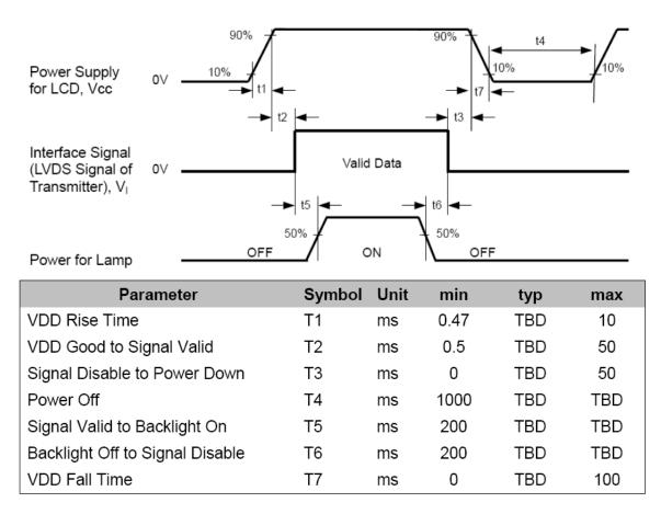
Note1: When VDD is on, but the value is lower than 4.5V, a protection circuit may work, then the module may not display.
