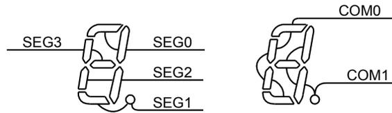
Figure 23-7 Example of COM and SEG Pin Connections
