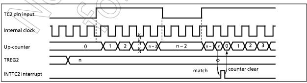
Figure 2-24. Window Mode Timing Chart
