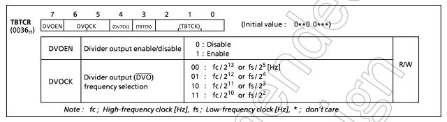
Figure 2-11. Divider Output Control Register
