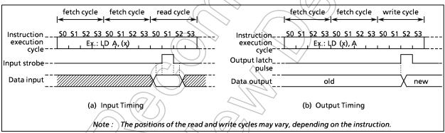
Figure 2-2. Input/Output Timing (Example)
