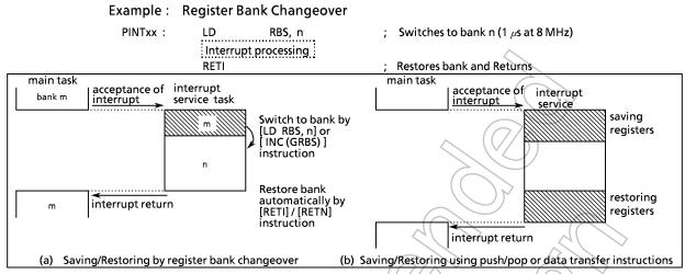
Figure 1-25. Saving/Restoring General-purpose Registers
