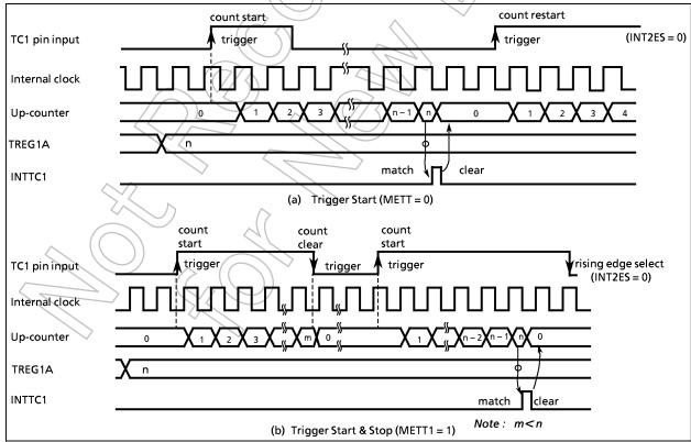
Figure 2-16. External Trigger Timer Mode Timing Chart
