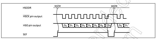
Figure 2-43. High-speed Serial Output Timing Chart
