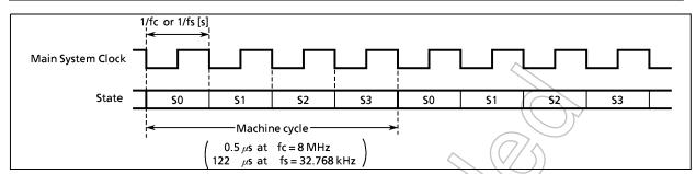
Figure 1-13. Machine Cycle
