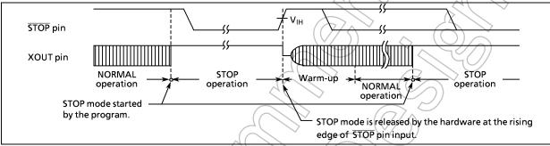
Figure 1-17. Edge-sensitive Release Mode
