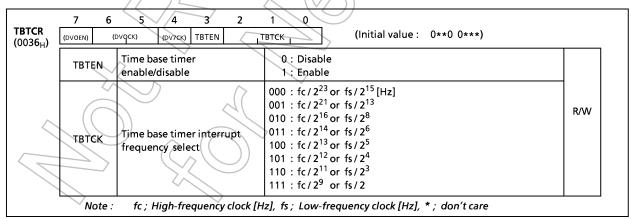
Figure 2-10. Time Base Timer and Divider Output Control Register
