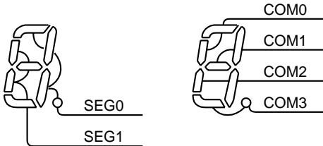
Figure 15-6 Example of COM, SEG Pin Connection (1/4 Duty)
