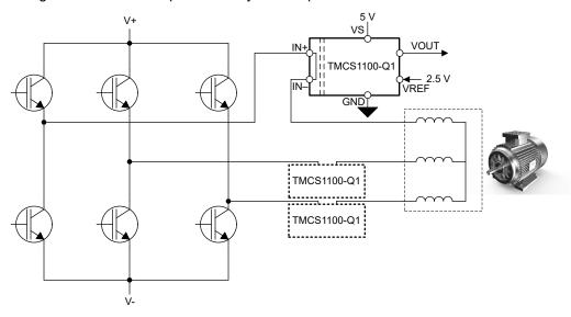
Figure 10-2. Inline Motor Phase Current Sensing
