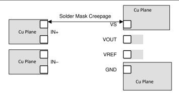
Figure 12-2. Layout for System Creepage Requirements
