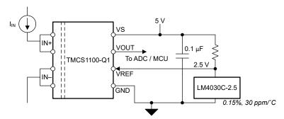
Figure 10-3. TMCS1100-Q1 Example Current-Sense System Design
