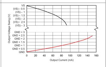
Figure 7-12. Output Swing vs. Output Current
