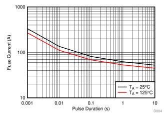
Figure 8-10. Single-Pulse Leadframe Capability
