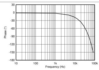
Figure 7-10. Phase vs. Frequency, All Gains
