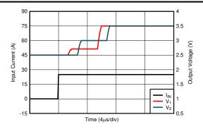
Figure 8-2. Transient Step Response
