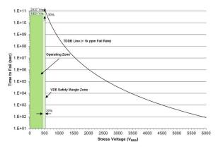
Figure 9-1. Insulation Lifetime
