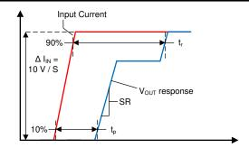
Figure 8-4. Current Overload Transient Response
