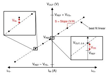
Figure 8-1. Sensitivity, Offset, and Nonlinearity Error
