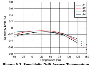
Figure 9-3. Sensitivity Drift Across Temperature
