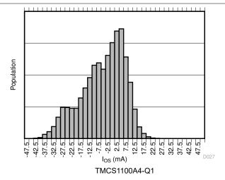
Figure 7-8. Input Offset Current Production Distribution
