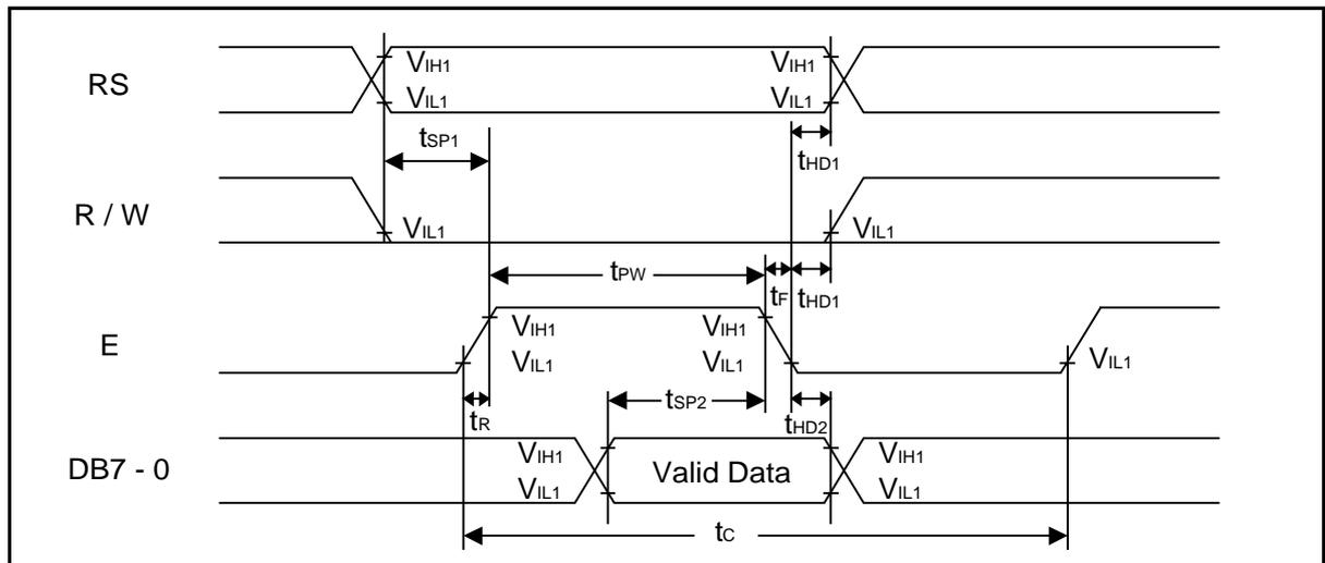
■ READ MODE ( Reading data from SPLC780A1 to MPU )
