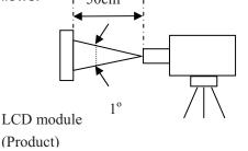
Luminance Meter (TOPCON BM-5A) Spectroradiometer(TOPCON SR-3)
