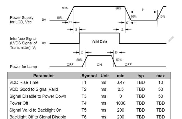
Note1: When VDD is on, but the value is lower than 4.5V, a protection circuit may work, then the module may not display.
