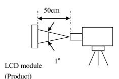
Luminance Meter (TOPCON BM-5A) Spectroradiometer(TOPCON SR-3)
