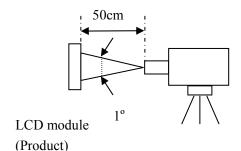
Luminance Meter (TOPCON BM-5A) Spectroradiometer (TOPCON SR-3)
