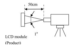
Luminance Meter (TOPCON BM-5A) Spectroradiometer(TOPCON SR-3)
