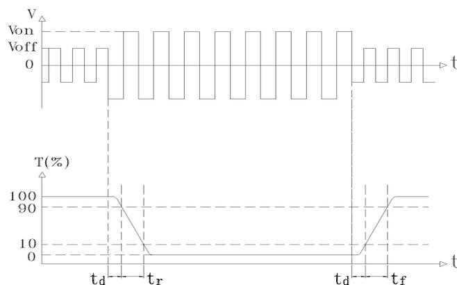
Turn on time:  $t_{on} = t_d + t_r$       Turn off time:  $t_{off} = t_d + t_f$
