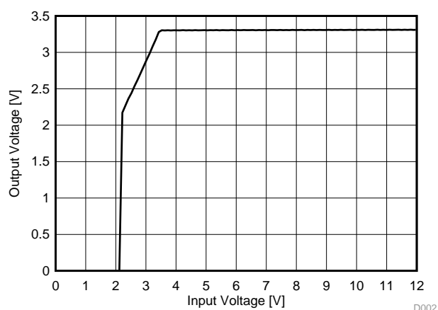
Figure 1. TLV2217-33 Output Voltage vs Input Voltage
