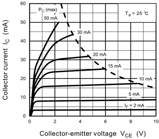
**Fig. 11.7  $I_C - V_{CE}$**
