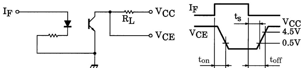
Fig. 10.1 Switching Time Test Circuit and Waveform
