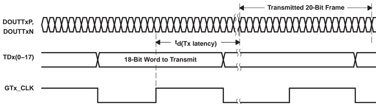
Figure 2. Transmitter Latency
