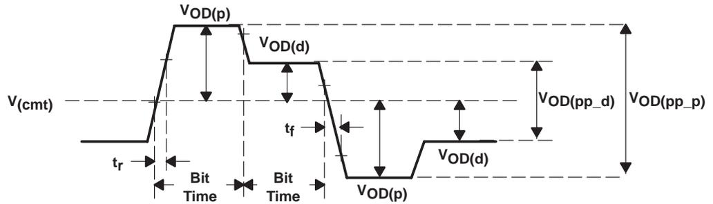
**Figure 8. Differential and Common-Mode Output Voltage Definitions**
