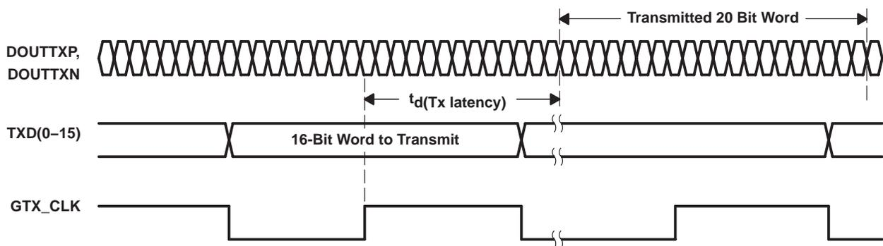
Figure 3. Transmitter Latency
