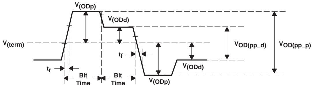
**Figure 12. Differential and Common-Mode Output Voltage Definitions**
