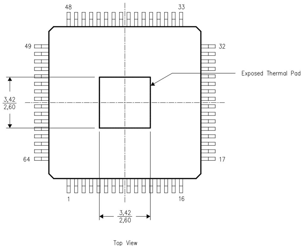
NOTE: All linear dimensions are in millimeters
