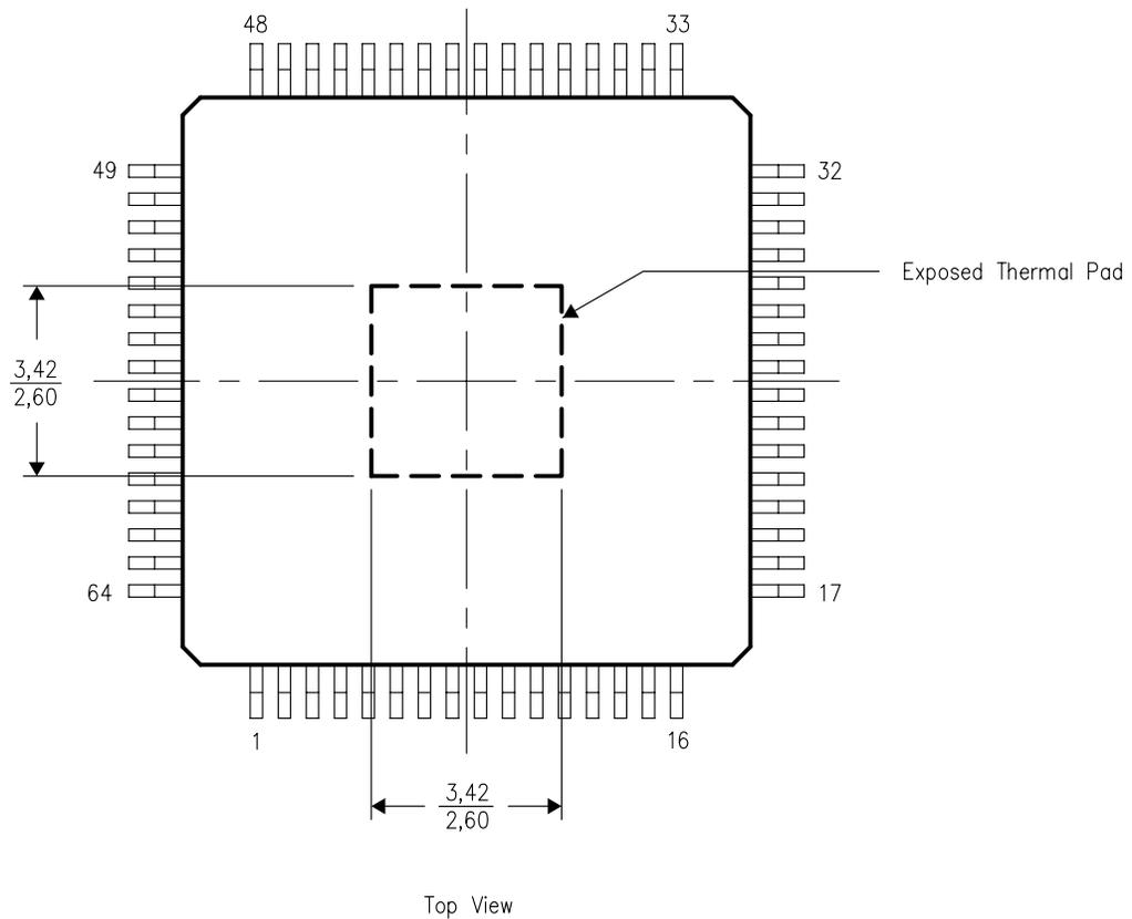
NOTE: All linear dimensions are in millimeters
