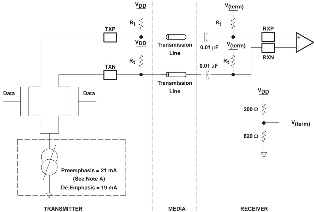
NOTE A: This assumes  $R_{REF} = 200 \Omega$  and termination resistance =  $50 \Omega$ . See Figure 14 and section *choosing  $R_{REF}$  resistor values* for more information.
