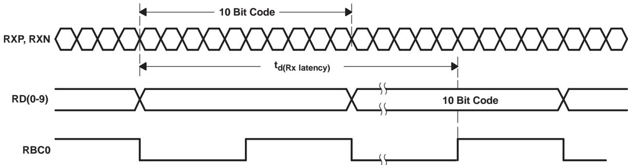
Figure 6. Receiver Latency - TBI Normal Mode Shown
