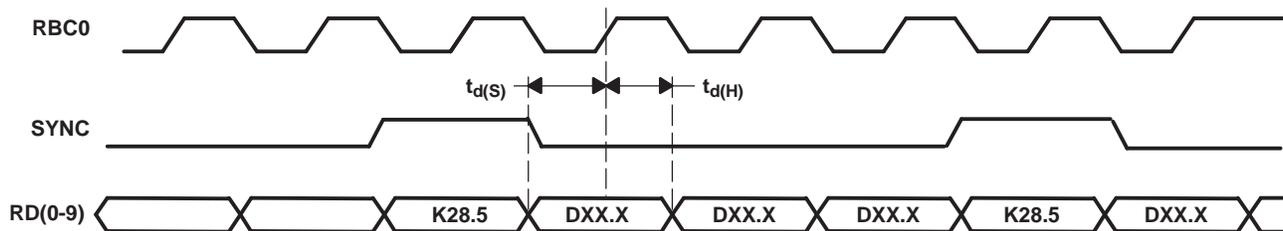
Figure 3. Synchronous Timing Characteristics Waveforms (TBI full-rate mode)
