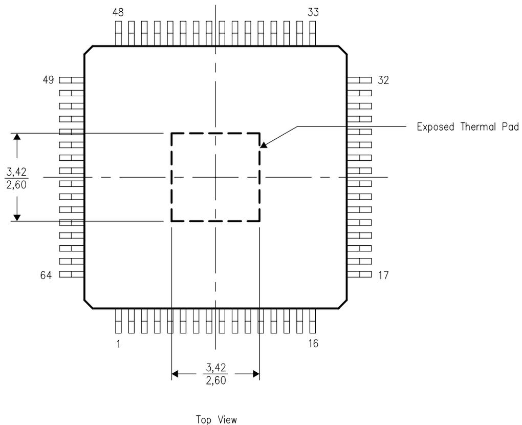
NOTE: All linear dimensions are in millimeters
