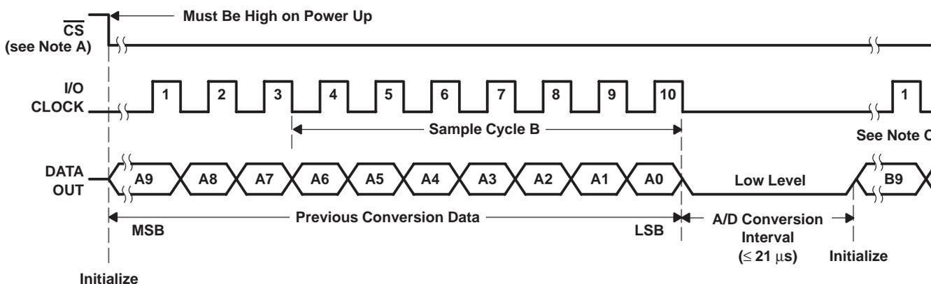
Figure 7. Timing for 10-Clock Transfer Not Using  $\overline{\text{CS}}$
