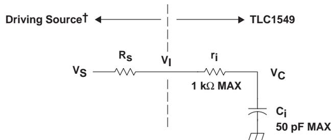
$V_I$  = Input Voltage at ANALOG IN
