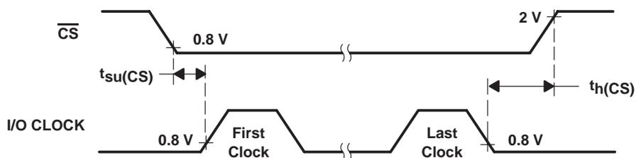
Figure 4. CS to I/O CLOCK Voltage Waveforms
