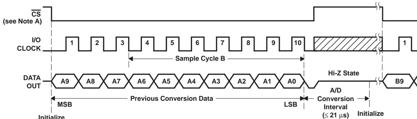
Figure 6. Timing for 10-Clock Transfer Using  $\overline{\text{CS}}$
