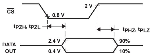
Figure 3. DATA OUT to Hi-Z Voltage Waveforms
