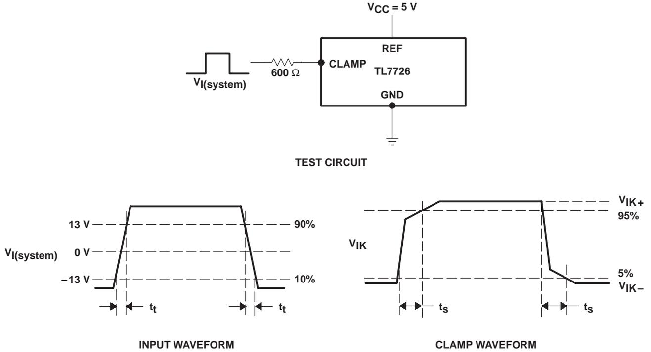
Figure 1. Switching Characteristics
