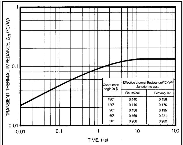
**Fig.8** Transient thermal impedance - junction to case
