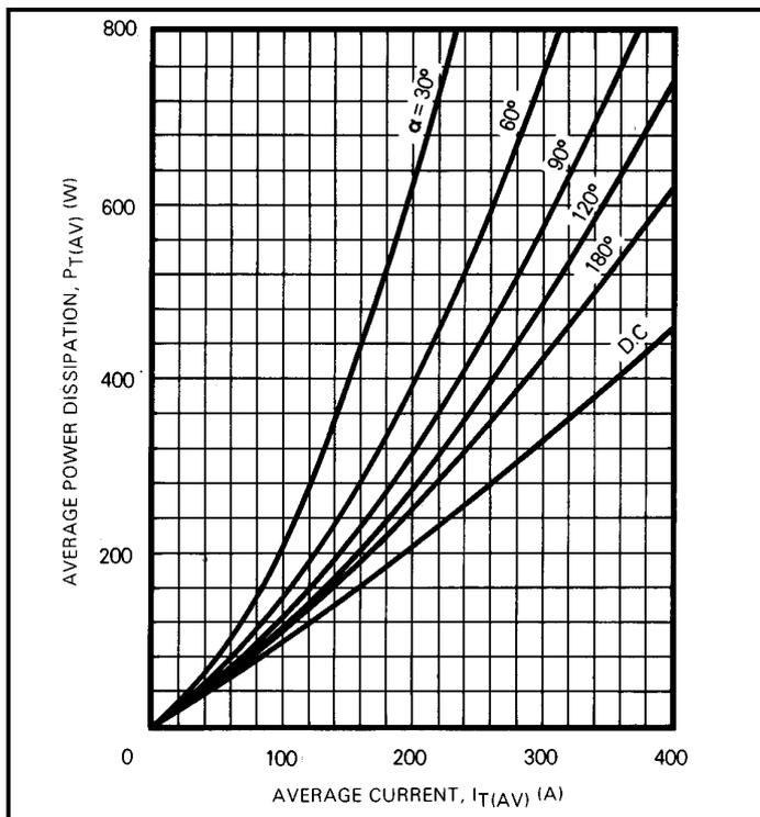
Fig.3 Maximum on-state power dissipation for sinusoidal current waveform
