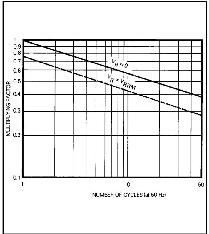
Fig.10 Multiplying factor for non-repetitive surge on-state current
