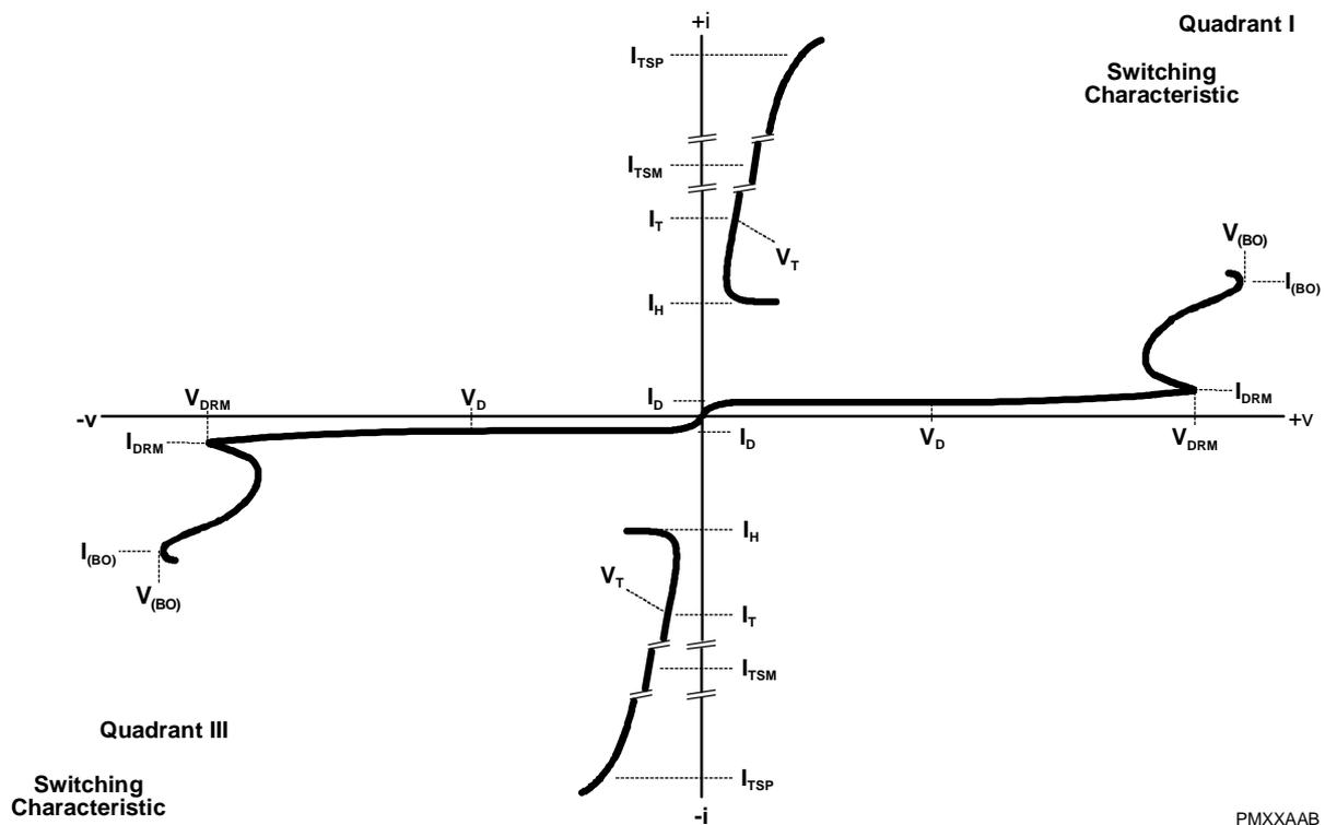
**Figure 1. VOLTAGE-CURRENT CHARACTERISTIC FOR T AND R TERMINALS
