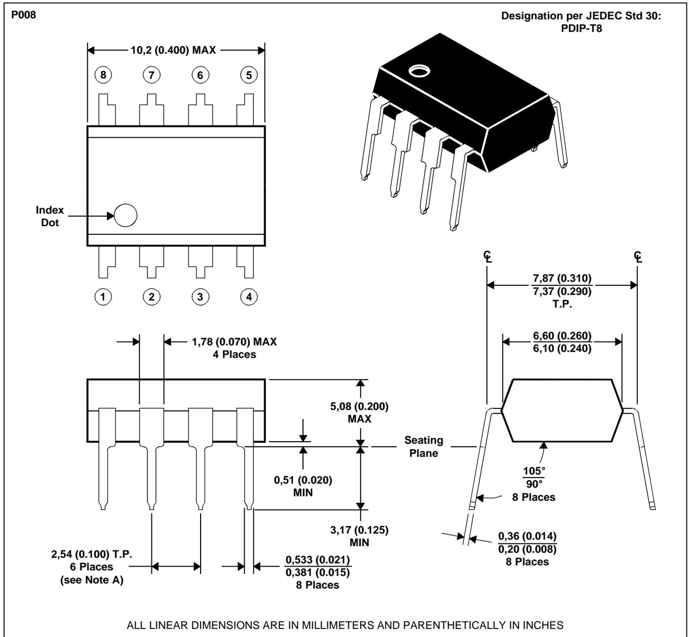
NOTE A: Each pin centerline is located within 0,25 (0.010) of its true longitudinal position
