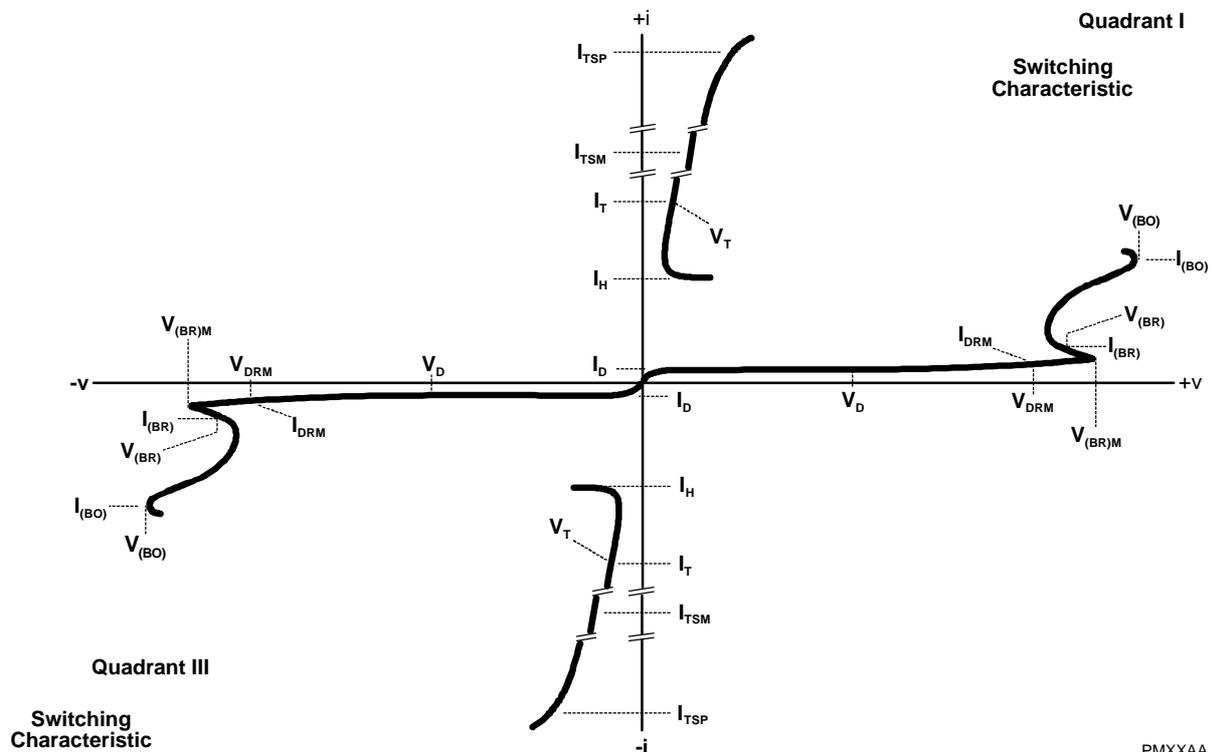
Figure 1. VOLTAGE-CURRENT CHARACTERISTIC FOR ANY PAIR OF TERMINALS
