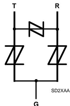
Terminals T, R and G correspond to the alternative line designators of A, B and C causes the device to crowbar. The high crowbar holding current prevents d.c. latchup as the current subsides.
