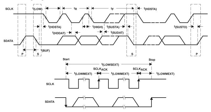
Figure 1. SMBus Timing Diagram
