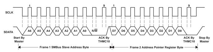
Figure 4. SMBus Timing Diagram for Send Byte Format (Used for One-Shot Command)
