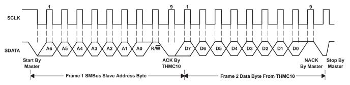
Figure 5. SMBus Timing Diagram for Recieve Byte Format
