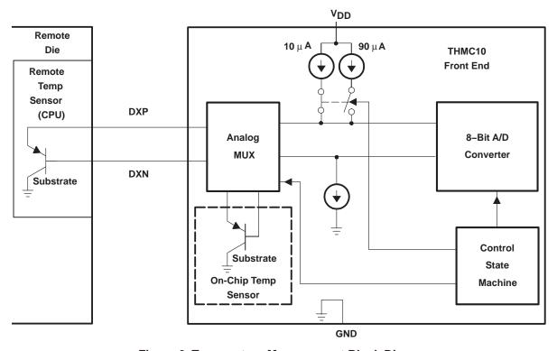
Figure 6. Temperature Measurement Block Diagram
