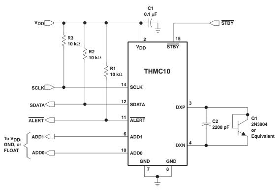
Figure 8. Typical Application Schematic
