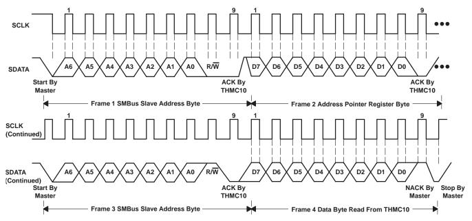
Figure 3. SMBus Timing Diagram for Read Byte Format
