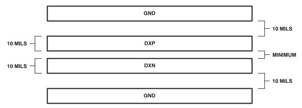
Figure 7. Recommended PC Board Layout for DXP/DXN Traces
