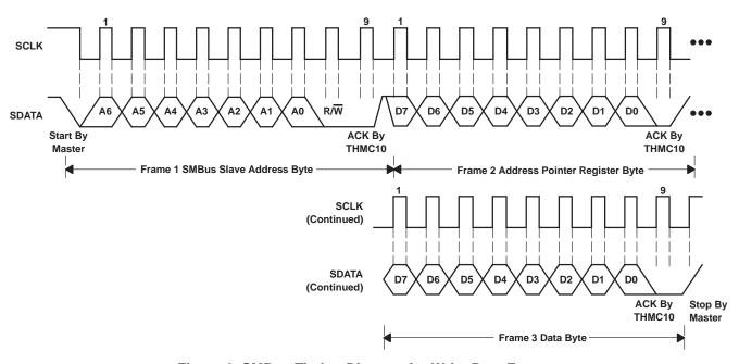
Figure 2. SMBus Timing Diagram for Write Byte Format
