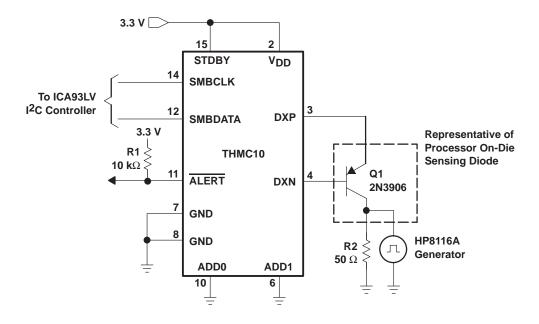
NOTE: No 0.1  $\mu$ F V<sub>DD</sub> capacitor. No 2200 pF DXP-DXN filter capacitor.
