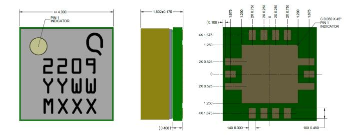
UNLESS OTHERWISE SPECIFIED DIMENSIONS ARE IN MILLIMETERS. TOLERANCE IS: .XX =  $\pm 0.25$ ; .XXX =  $\pm 0.127$ , and ANGLES =  $0.5^{\circ}$
