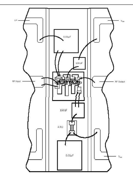
RF connections: Bond using two 1-mil diameter, 20 to 30-mil-length gold bond wires at RF Input and one 1-mil diameter, 20 to 30-mil-length gold bond wire at RF Output for optimum RF performance.
