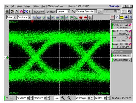
Photodiode Current = 9.5 uA RMS
