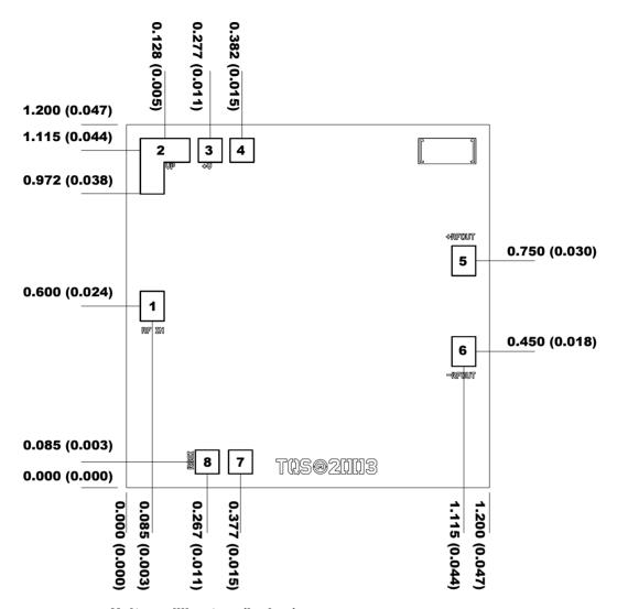
Units: millimeters (inches) Thickness: 0.100 (0.004)
