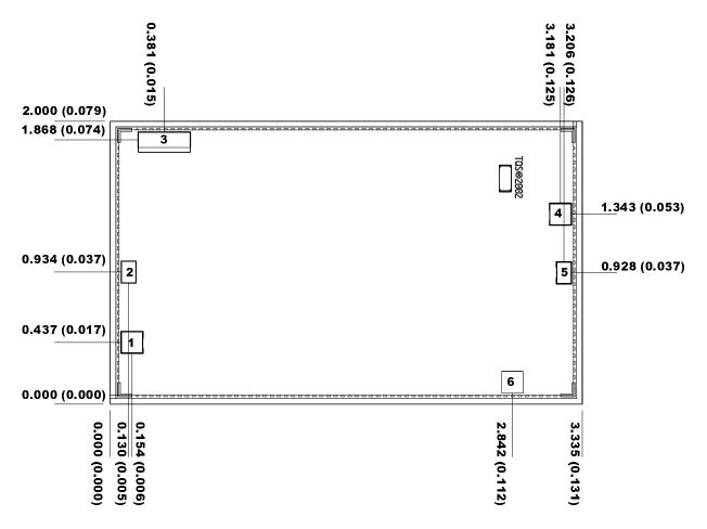
Units: millimeters (inches) Thickness: 0.100 (0.004)
