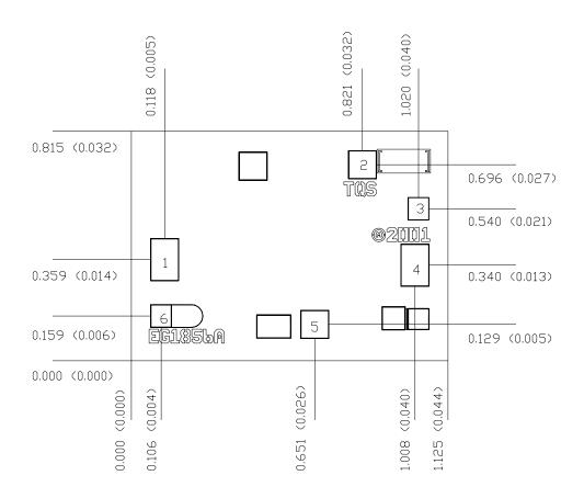
Units: millimeters (inches) Thickness: 0.1016 (0.004)
