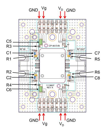
NOTE: Both Top and Bottom Vd and Vg must be biased.
