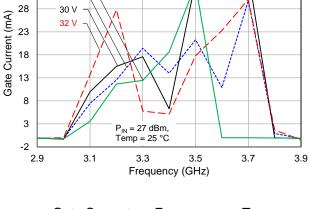
Gate Current vs. Frequency vs. V<sub>D</sub>
