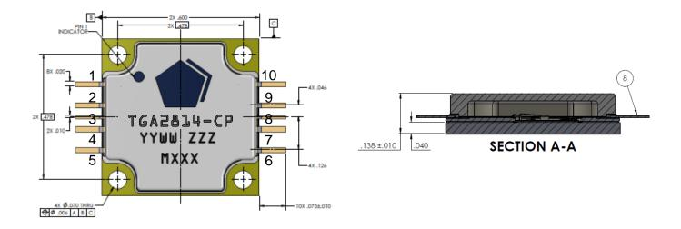
Units: inches Tolerances: unless specified  $x.xx = \pm 0.01$   $x.xxx = \pm 0.005$ Materials: Base: Copper Lid: Plastic All metalized features are gold plated Part is epoxy sealed Marking: 2814: Part number YY: Part Assembly year WW: Part Assembly week ZZZ: Serial Number MXXX: Batch ID
