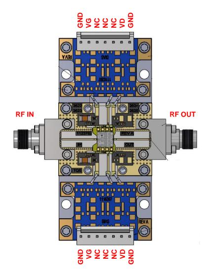
PCB is made from Rogers 4003C dielectric, .008 inch thick, 0.5 oz. copper both sides.
