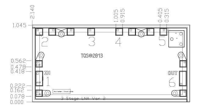
Units: millimeters Thickness: 0.10 Die x,y size tolerance:  $\pm$  0.050 Ground is backside of die RF<sub>IN</sub> and RF<sub>OUT</sub> pads are symmetric
