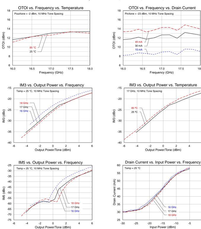
Conditions unless otherwise specified:  $V_D = 3 \text{ V}$ ,  $I_{DQ} = 30 \text{ mA}$ ,  $V_G = -0.6 \text{ V}$ , CW
