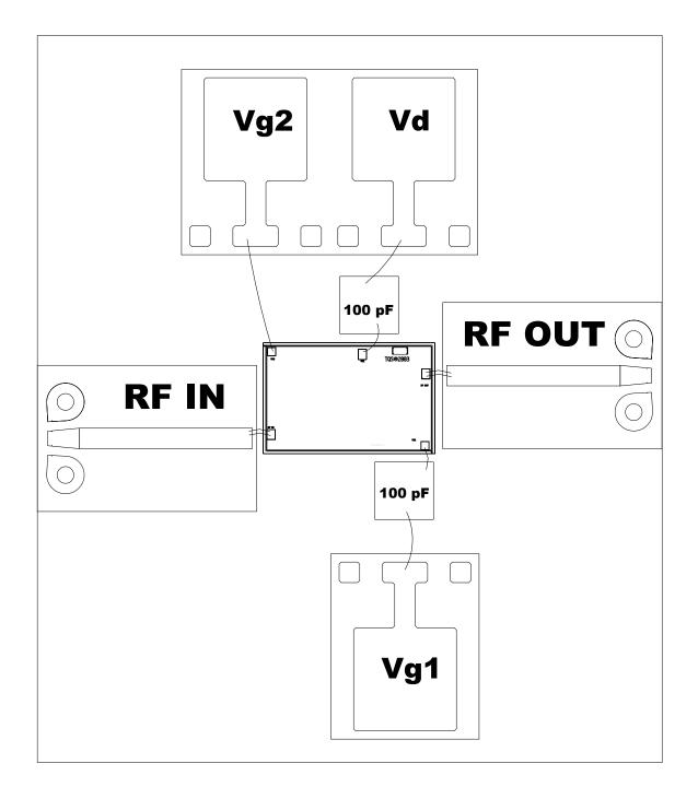
GaAs MMIC devices are susceptible to damage from Electrostatic Discharge. Proper precautions should be observed during handling, assembly and test.
