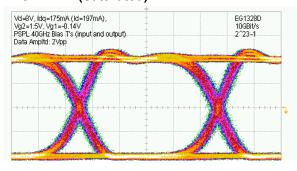
10GBit/s Performance Output = 8V P-P, Input = 2V P-P scale 2V/div, 20ps/div
