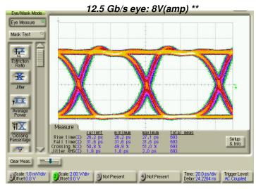
\*\* Input 12.5Gb/s data stream generated using an Anritsu PPG (Vin=2Vpp).
