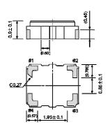
Pin map Connection Pin VC-TCXO TCXO N.C 2 GND 3 OUT Vcc
