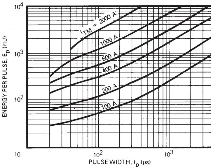
FIG. 15 ENERGY PER PULSE FOR TRAPEZOIDAL PULSES
