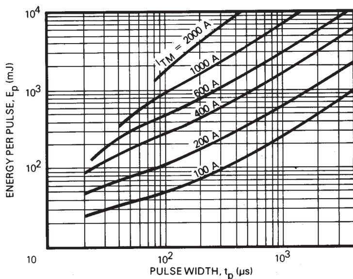
FIG. 12 ENERGY PER PULSE FOR TRAPEZOIDAL PULSES
