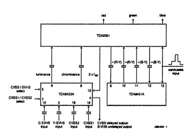
Fig.2 PAL decoder configuration.
