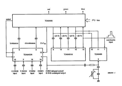
Fig.3 PAL-NTSC-SECAM decoder configuration.
