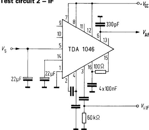
Block diagram and application circuit
