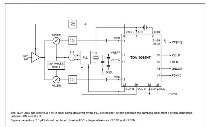
Fig.3 Front-end receiver schematic.
