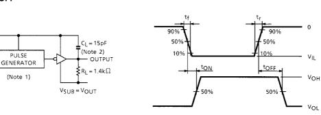
Note 1: Pulse width 50  $\mu$ s, Duty Cycle 10% Output Impedance 50  $\Omega$ , t<sub>r</sub> ≤ 10 ns, t<sub>f</sub> ≤ 5 ns Note 2: C<sub>L</sub> includes probe and jig capacitance.
