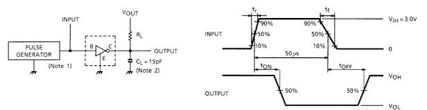
Note 1: Pulse width 50  $\mu$ s, Duty Cycle 10% Output Impedance 50  $\Omega$ , t<sub>f</sub> ≤ 5 ns, t<sub>f</sub> ≤ 10 ns Note 2: C<sub>L</sub> includes probe and jig capacitance.
