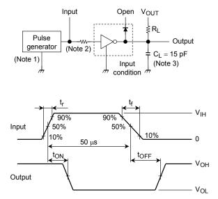
Note 1: Pulse width 50  $\mu$ s, duty cycle 10% Output impedance 50  $\Omega$ , t<sub>r</sub> ≤ 5 ns, t<sub>f</sub> ≤ 10 ns
