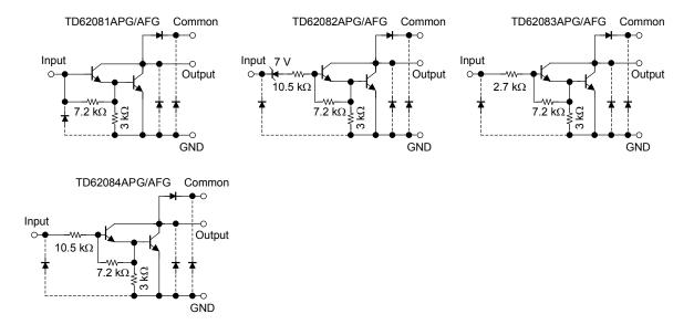
Note: The input and output parasitic diodes cannot be used as clamp diodes.
