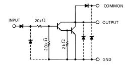
Note: The input and output parasitic diodes cannot be used as clamp diodes.
