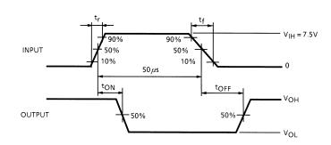
Note 1: Pulse Width 50  $\mu s$ , Duty Cycle 10% Output Impedance 50  $\Omega$ ,  $t_{r} \le 5$  ns,
